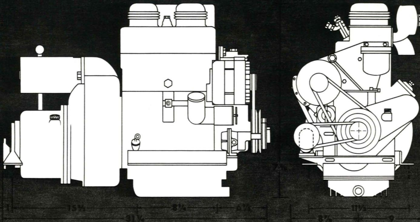
**TYPE** 2-cylinder, 4-cycle, vertical in-line diesel. Over-head valves. Direct injection.
